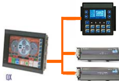
Figure 1 – High Availability System XLe as Master, QX as Slave, and SmartStix I/O
